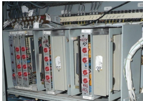
Fig5: Final Regulator Supply Cards
