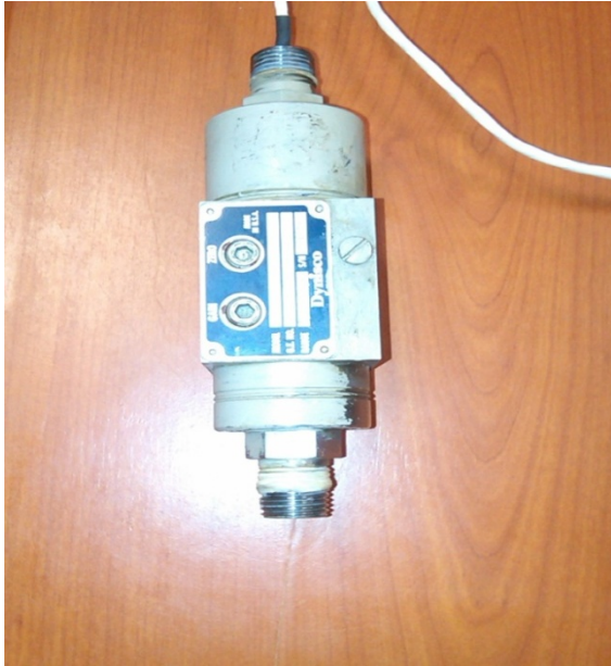
Fig14: Faulty Fuel Gas Transmitter 96FG
